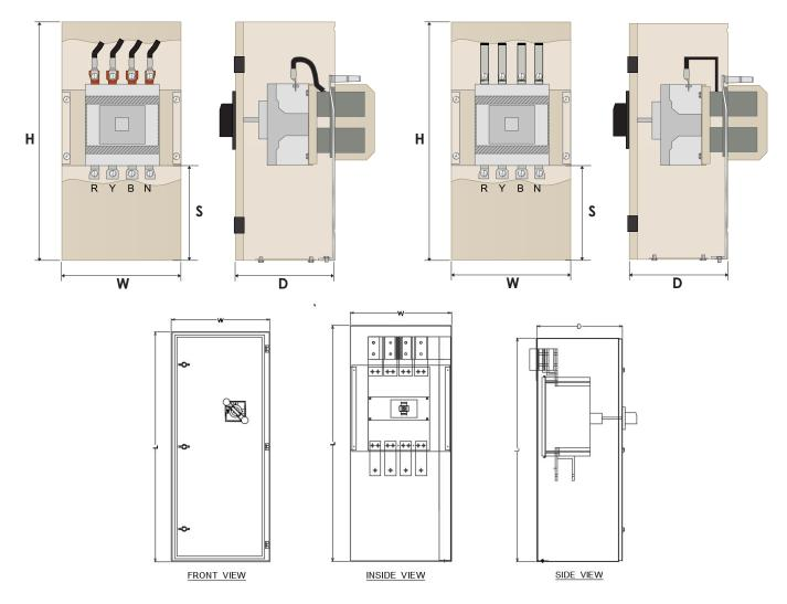
Wilmar Busway offers a range of tap off units to fit all ranges for multiple applications. All Plug-in & Tap-off Units are suitable for MCCB.
