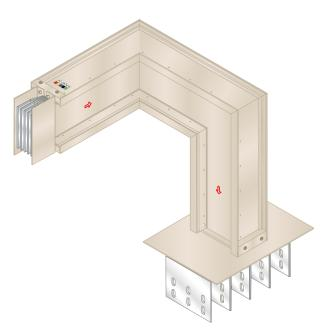
True Sandwich Design achieved with the help of precise extruded housing and perfectly insulated conductors, eliminate pathways for propagation of Flame, Gas, Smoke referred to as "Chimney Effect", thus making Sandwich Busways Safer.
