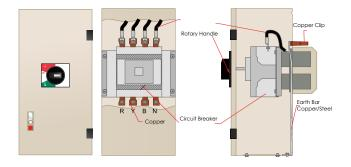
The unit is also supplied with all connections and accessories to ensure the connection to the outgoing cable termination are correctly and safely achieved.
