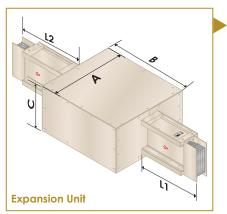
building expansion joint. Long straight runs where both ends are connected in fixed position also require expansion joints. Flexible conductors inside the expansion joint allow/ accommodate movement caused due to expansion and contraction of busway system.
