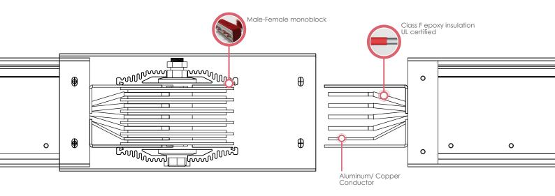
Unique two piece IP65 aluminum trunking case TESTED
